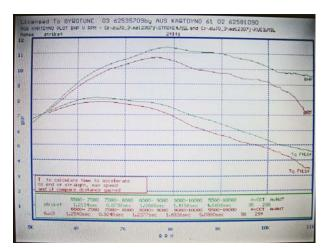
The cylinder was compared to 3 cylinders, the first one shown on the left shows the STRIKE cylinder (green line) compared to a "very average" Yamaha J cylinder (red line). The difference is very obvious.
