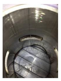
The first shows a Comer cylinder where the roof of the exhaust port has been "peened" in an attempt to raise the port. With a layer of carbon over this, it would be difficult to detect this illegal modification.
