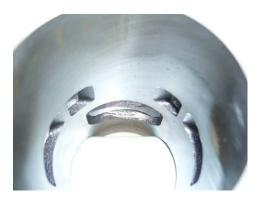
The second shows a KT100S cylinder that has had some excessive (illegal) grinding, on the base of the inlet port, presumably to clean up some surface imperfections.
